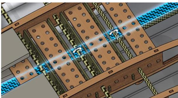
The aircraft's structure has been designed in a manner that allows for the main section of the fuselage and the wing to be detached from the main fuselage strut and tail section as shown.
