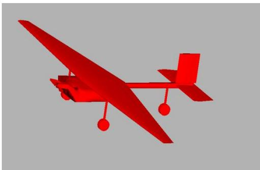
Secondly, the aircraft was tested for stability and control in X-Plane Simulation Software. This test revealed that our aircraft needs a slightly bigger wing span, and a much larger tail and fin.
