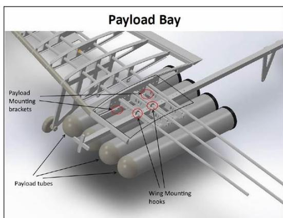
thin glass fibre . It will be mounted directly to fuselage. There is no fuselage in traditional way; it is just square tube made out of carbon fibre. In this way the drag should be kept at minimum to improve the aircraft performance. At initial stage we are aiming for 6 tennis balls in each tube, times
