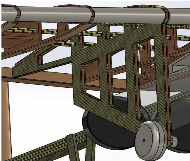
was selected in order to produce a structure that was both relatively easy to manufacture while increasing the structural integrity of the component over that of an equivalently dimensioned plywood only design.
