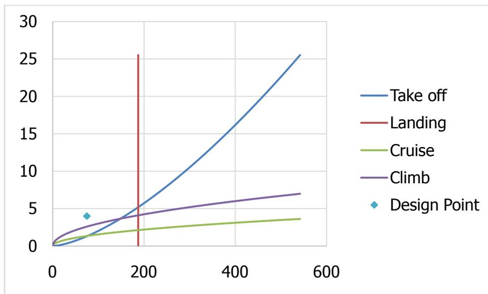
We used these constraints as a basis for our UAV design. Once we generated ideas we then finalised the design in such a way as to fit these constraints using them as
