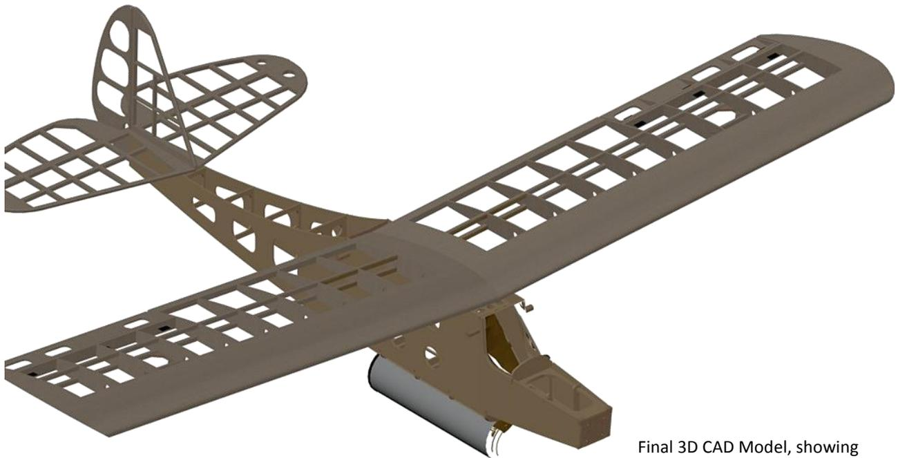
Final 3D CAD Model, showing bare airframe
